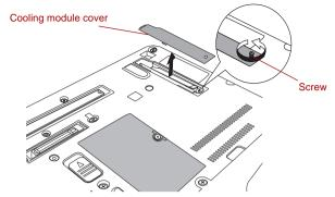
Figure G-1 Removing the cooling module cover
